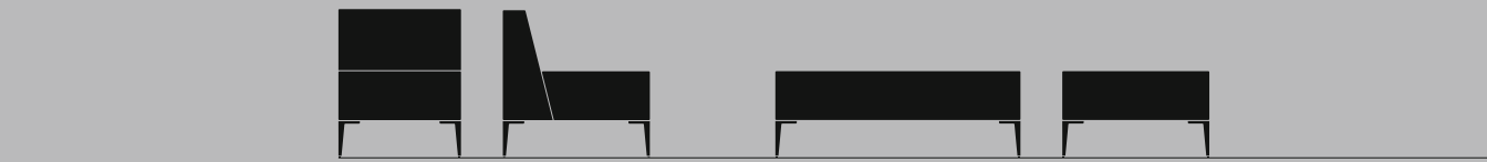
Módulo individual Modulo individual Single seat module Module 1 place Banco Banco Bench Banc H 713 L 600 P 703 H 413 L 1200 P 703
